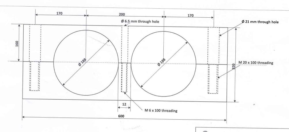
Note: All Dim in MM Plate Thickness : 30mm MOC : MS
